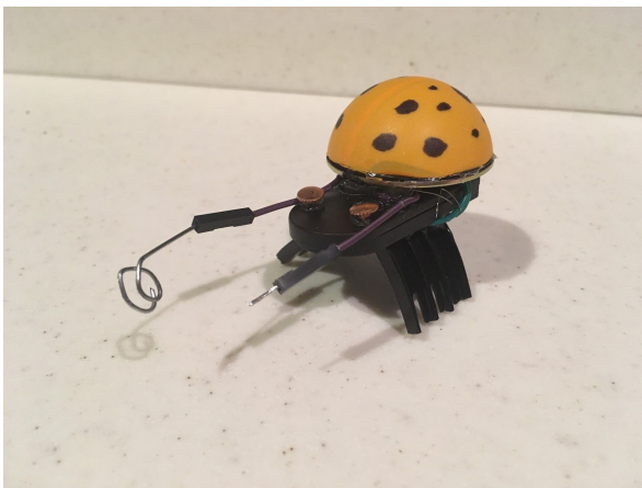
Fig 5. The humbug uses the simplest way to create sound using a speaker, it does so by manually closing the circuit using the two metallic heads of the wires.
