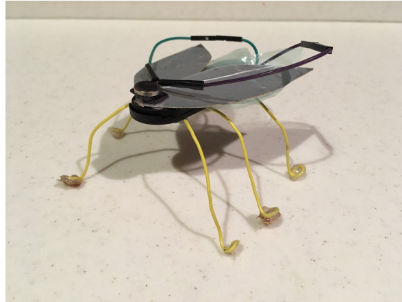
Fig 4. The pond skater bug went through several tests in order to find a good material for the legs to support the bug in the water. This prototype after many trials did not work consistently and was removed from the kit.
